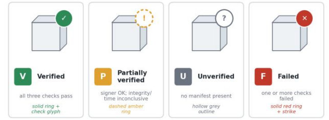
Fig. 2. Graduated trust-indicator set anchored to a spatial asset. Each badge couples a distinct color, glyph, and ring style to one of the four trust states; salience and modality are modulated at run time by the controller of Section IV.
